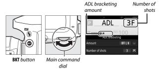
At settings other than zero, and BKT are displayed respectively in the control panel and viewfinder; a light icon and the bracketing amount appear in the information display.
