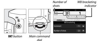
At settings other than zero, and and BKT are displayed respectively in the control panel and viewfinder; a weeking indicator appear in the information display.
